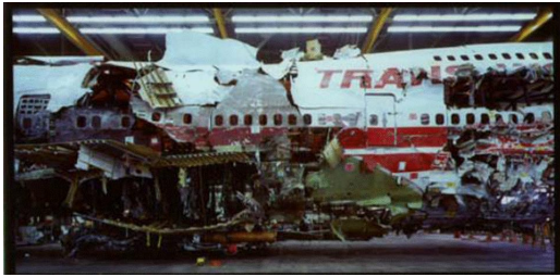
Figure 1 Re-constructed Wreckage of TWA flight 800
