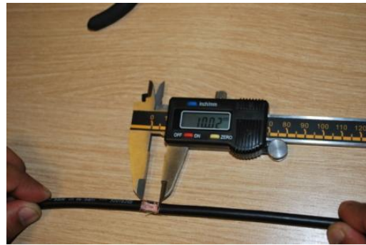
Figure 4. Coaxial cable with a 10 mm damage created on the shield and insulation on one side with the core conductor undamaged. The fault was created at around 2 meters from the end of a 6 meter long cable.
