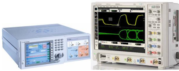
Figure 3 Agilent 3.35 GHz pattern generator and 4 GHz 20 GS/s Infiniium oscilloscope used for the development of the ETDR technique.
