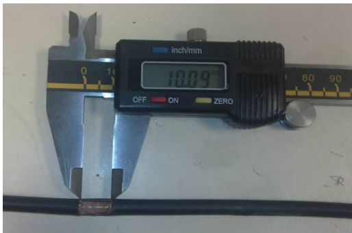
Figure 4 Coaxial cable with a 10 mm damage created on the shield and insulation on one side with the core conductor undamaged. The fault was created near the middle of a 6 meter long cable.
