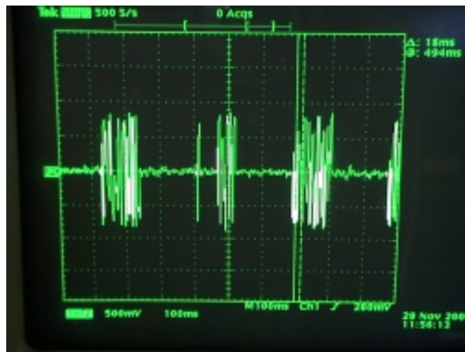
Figure 5. The output from the oscilloscope showing the PLC message as it is being transmitted along the DC power line. The oscilloscope is coupled to the AC signal so that the DC offset is not shown. An inherent error has also occurred in the message transmission.
