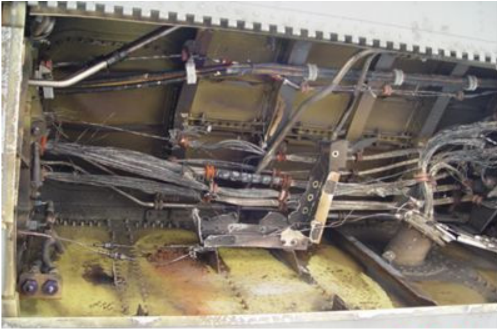
Figure 2. In-flight electrical/hydraulic fire in an aircraft wing area. The fire caused extensive wiring damage, a fire extinguisher system to rupture, and damage to the wing structure.
