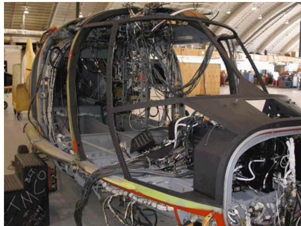
Figure 1: HH-65 DIT-MCO Testing
